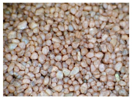
The particle shape is predominantly **C3** which is round, low sphericity.
